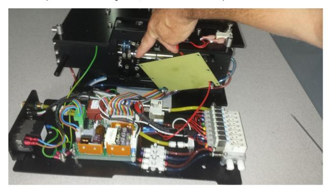
There is an pneumatic fitting assembly here with blanking screws, check here to ensure no air leak present in this area.
