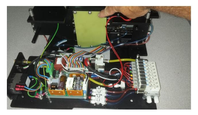
Remove this panel to access air fitting behind, Be careful do not lose the spacer bar fitted!
