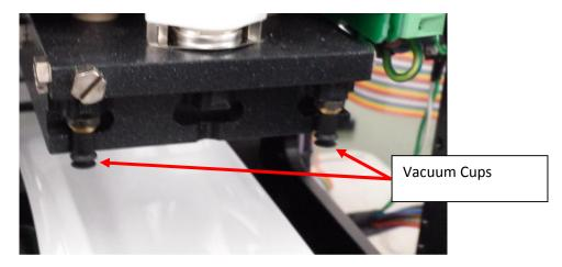
The vacuum cups must be of good condition to enable accurate and reliable foil/film pick up to continue with the sealing action of the Wasp plate sealer.
