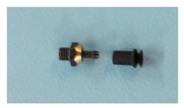
Visually Inspect the Vacuum cup ensuring the 'sealing lip' of each vacuum cup is complete and not damaged.
