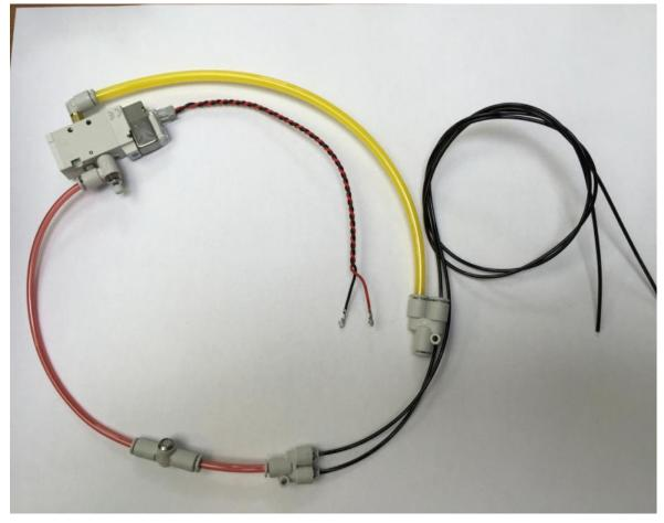
Replace the red air pipe (between the flow controller fitted to the solenoid valve and the 4mm to 2mm Y fitting) with the supplied parts, the inline flow controller locates where the original inline quick exhaust valve is fitted (fixed to the side plate using a p-clip).
