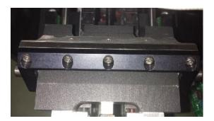
With light finger pressure push down on gripper face, and retighten retaining screws.
