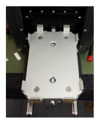
Locate Front gripper, with pneumatic services ON, release the m3 retaining screws that attach gripper face to gripper back plate.
