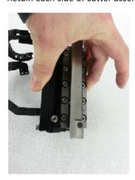
Apply a gradual pressure to front cutter Die, and tighten retaining screws.
