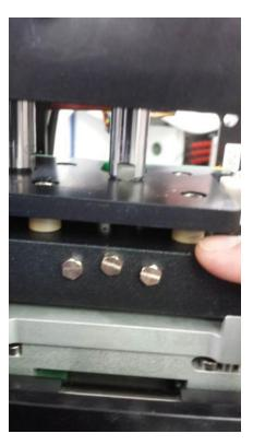
11. CAREFULLY withdraw the heater block assembly which will retain the thermocouple internal to block & heater cartridges wired to heater connection board.
