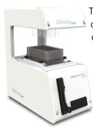
The Ultravap Mini blowdown evaporator is purpose designed for low usage research and development departments where low numbers of individual plates or vials need drying. The Ultravap Mini is simple to operate and maintain. Installation requires only connection to a gas supply and standard mains socket. With manual control of the needle depth, gas temperature and flow rate, it allows fine control and quicker drying times than other standard methods.
